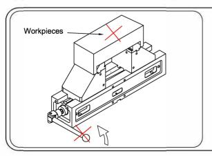
Usually turn handle clockwise when clamping work.
