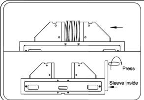
In order to avoid distortion, in the case of thin walled, hollow or lower rigidity workpieces, set the desired clamping rage before performing the suffcient preliminary clamping by turning the handle clockwise, pushing the sleeve forward as shown in the firure.
