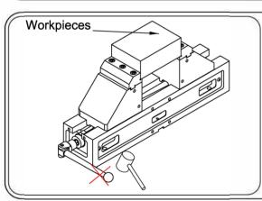
Caution when operaling; The design of the vise with its active handle can create over one time of clamping force than general vise does. Do not hit the handle or its vicinity with a hammer ect., while fastening.
